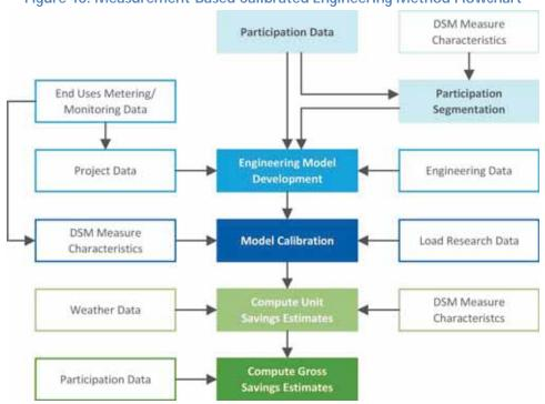
Figure 46. Measurement-Based Calibrated Engineering Method Flowchart
