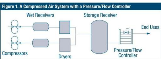
Compressed Air System with a Pressure/Flow Controller<sup>3</sup>
