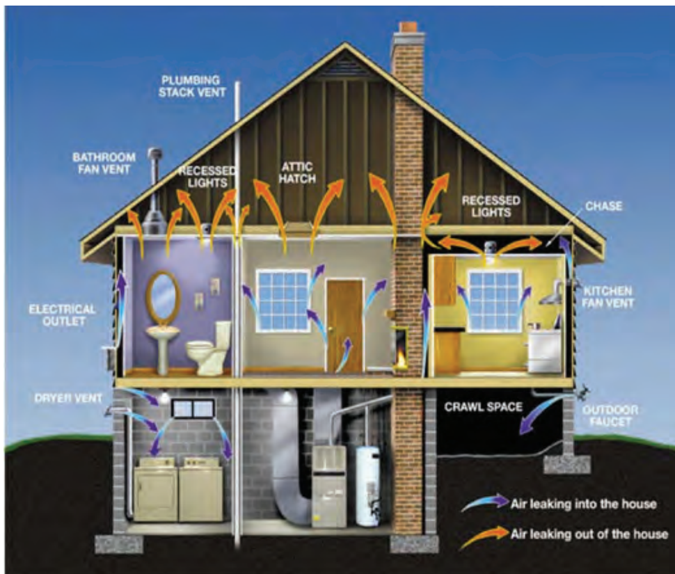
Diagram of general air leakage paths.
